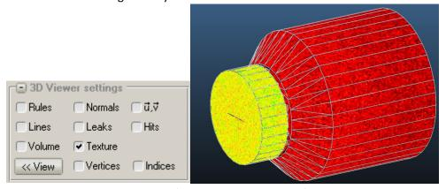
• In the advanced viewer options (click the << View button), you can choose to render only the back side of facets, which will allow to peek inside the geometry:
