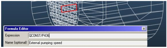
Explanation: QCONST is the outgassing, P436 is the pressure on facet #436 (in red)
