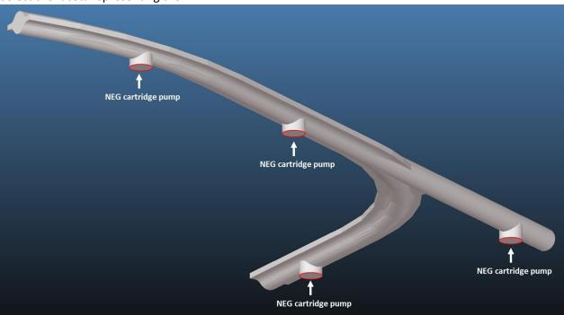
On the right side, enter the previously calculated 25 l/s pumping speed (if you select the 4 pumps together, you can only edit the sticking factor, enter 0.069 which will correspond to a total of 100 l/s pumping speed):
