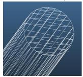
• We can fix the problem by **projecting** all triangles onto the facet's plane. Select the triangles and open the Mirror / Project command:
