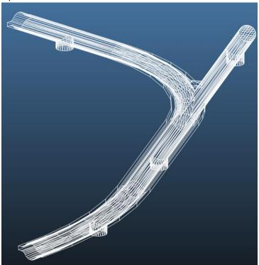
• We'll see that the end of the light extraction didn't collapse. This is a common problem of using STL files, and its cause is that the CAD program exports coordinates with finite precision, and merging these triangles would create a non-planar facet.
