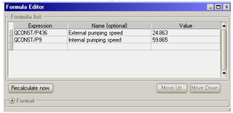
Explanation: QCONST is the outgassing, P436 is the pressure on facet #436 (in red)
