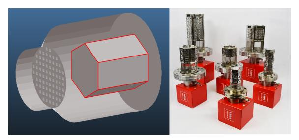
In this, first part we will approximate the effective (local) pumping speed of a NEG cartridge pump's pumping port. The goal is to use this result in the second part, when we'll be simulating a part of an accelerator.
