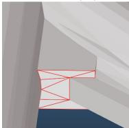
• And set an area-dependent outgassing of 1E-3 mbar.l/s/cm<sup>2</sup>:
